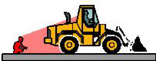
Blind Spot for a Front End Loader
